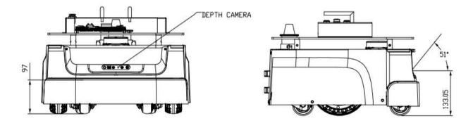
There is a deep camera on the chassis, which requires a certain clearance area to avoid being shielded or interfered;
