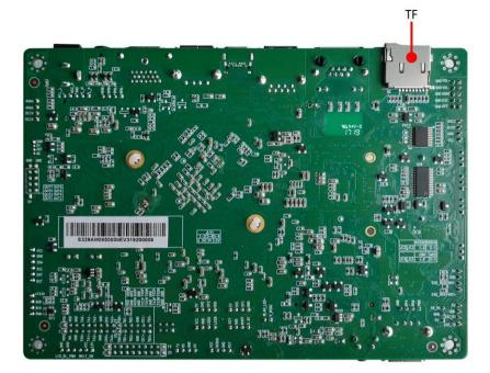
Caution : The identification method of the first pin on the main board is: 1 has a white and bold silkscreen; 2 the pins seen on the back of the main board are square holes.
