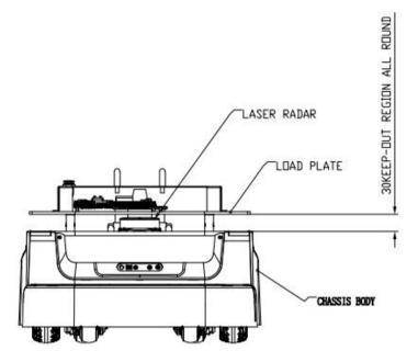
There is a radar between the chassis body and the host computer, which requires a certain clearance area to avoid being shielded or interfered;
