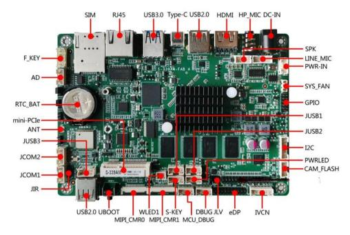
(2) Front IO diagram of the main board
