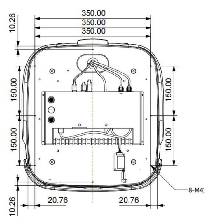
As shown in the figure above, there are a total of 8 M3 threaded holes for the installation and fixation of the host computer.
